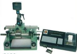
Computer Aided Setting System for accurate machine pre-setting from the toolroom.
